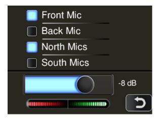
Note - Many Ivie controls can be configured in multiple ways in the Sonata<sup>TM</sup> and Aria<sup>TM</sup> programming software. This example of the RMI-4 has 4 independent buttons, but could just as easily be programmed with a 4 position selector instead. How to match and configure controls will be addressed in the next section.
