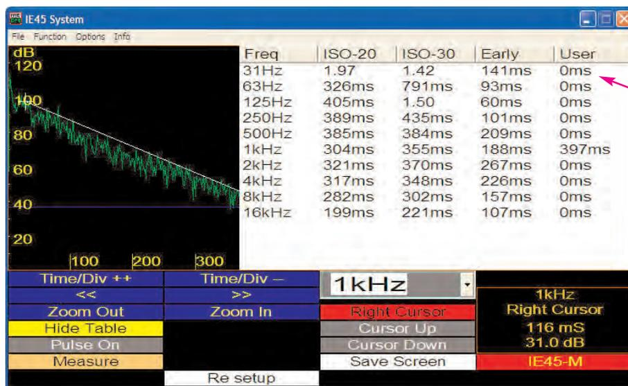
**Note:** Numeric measurement data is displayed for octave channels, or 1/3 octave channels, depending on whether you selected octave, or 1/3 octave RT60 measurements.
