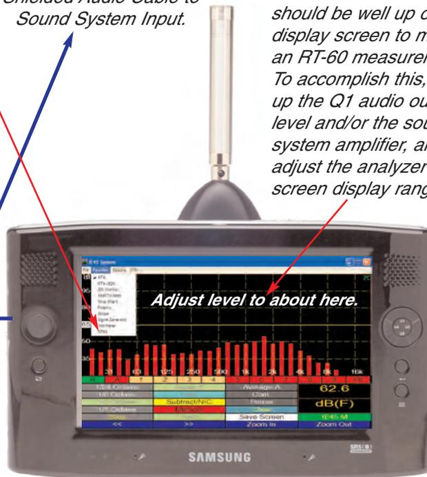
As can be seen, making a Pink Noise Mode RT60 measurement is easy and straight forward. Now, let's look at the steps required to make an Impulse Mode RT60 measurement. Next, we'll examine the results of an RT60 measurement. The measurement data gathering and formatting is the same for either mode of measurement.
