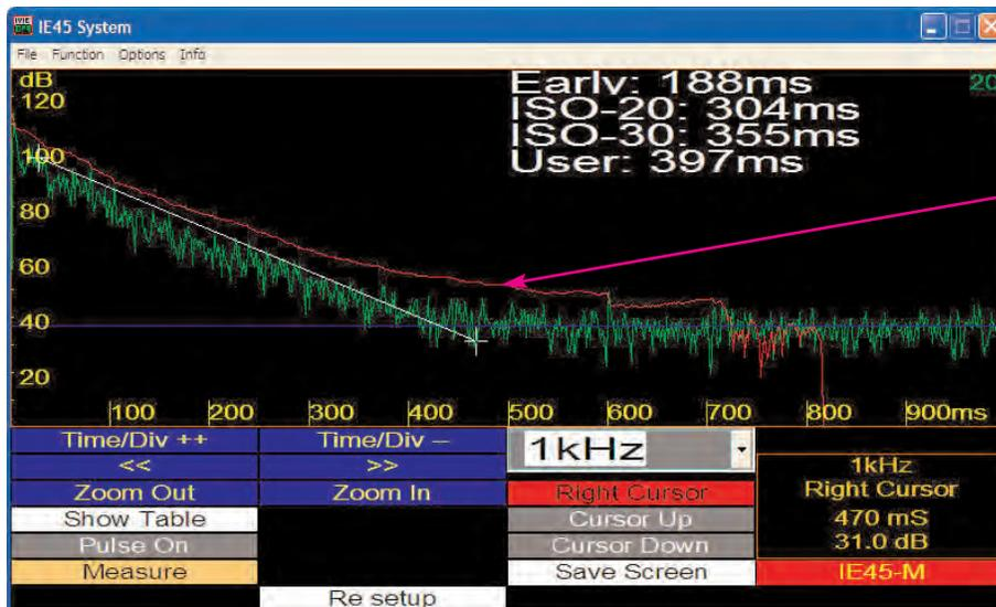
**Note:** The Schroeder curve is the decay curve with a smoothing algorithm applied. The left and right cursors can be placed on it, instead of the decay curve, to calculate RT60, if desired.
