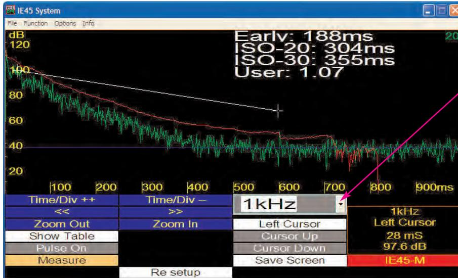
**Note:** Tapping here pops up a window which allows you to select for viewing the decay curve for any octave, or 1/3 octave channel. The default display channel is 1 kHz.
