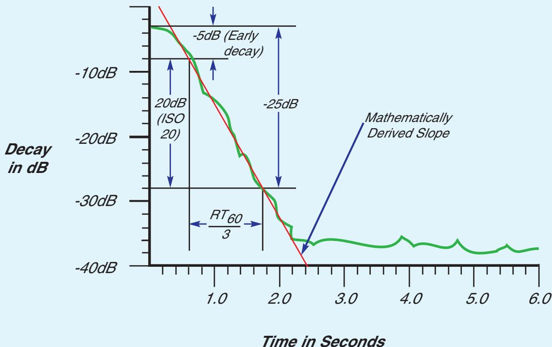
The above plot shows a decay curve and identifies sections of that decay curve. To insure statistical accuracy in measuring and plotting decay, the IE-35 and IE-45 take samples (of amplitude in dB) at the rate of 100 samples per second, regardless of the length of the measurement window selected.
