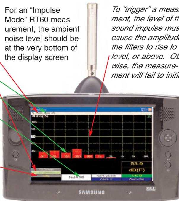
Proper selection of the measurement time window (Step 3) will assure the optimum view of the decay curve (not too steep
