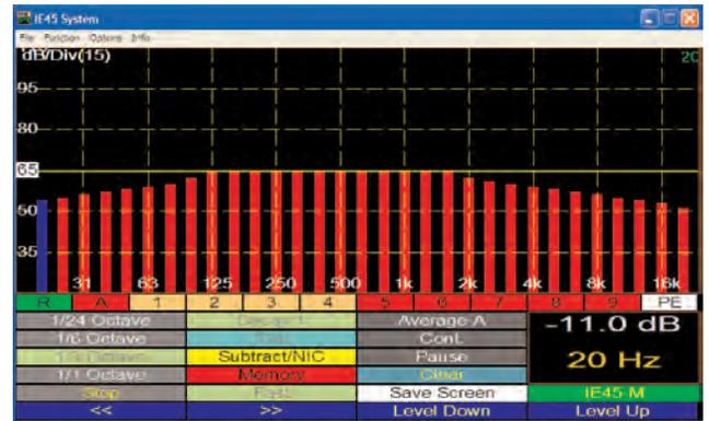
Step 3: Tap the "PT" Button to display the Preferred Curve Overlay. To turn off the Preferred Curve Overlay, tap the green PT Button. To edit the curve, tap the buff colored PT button. Tapping the white PT Button will again display the edited Preferred Curve.
