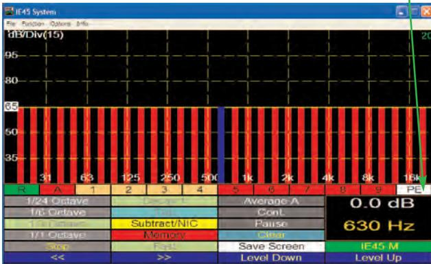
Step 2: Use the Joystick Left/Right, or the stylus to select frequency (blue bar) and the Joystick Up/Down to set amplitude until the curve entry is complete.
