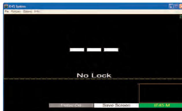
In the example screen above, the IE-45 is unable to achieve a “lock” on the signal. Make certain the pulse signal level is at least 10 dB above ambient. Move the microphone closer to the speaker.
