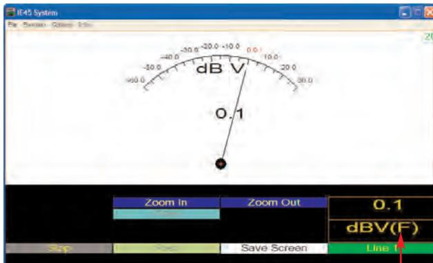
Measuring in dBV (dB relative to 1 volt rms).
