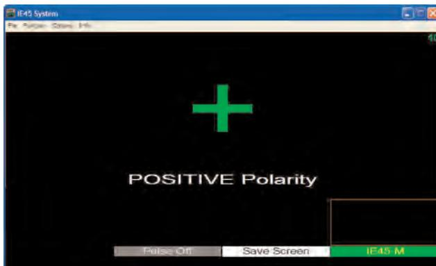
In the example screen above, the IE-45 has “locked” on the signal and identified the polarity of the signal as “Positive.”
