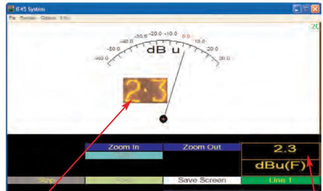
Measuring in dBu (dB relative to .775 volts rms).
