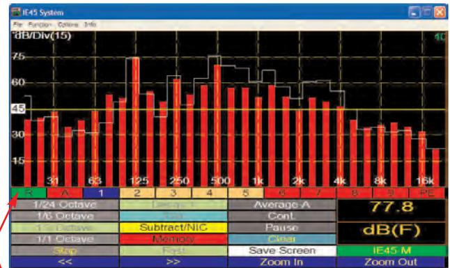
From left to right, the row of memory and display associated stylus buttons mean: R = Green; RTA display active. A = Red; Average display not on. 1 = Blue; data in memory being displayed. 2 - 5 = Buff; data in memory, but not displayed. 6 - 9 = Red; memories empty. PE = Red; no data in Preferred Curve Entry memory.
