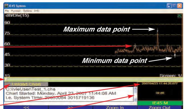
Scroll through data including: File name, Test date/time, Total number of data points, Sample interval, Weighting, Maximum SPL and time and Minimum SPL and time.
