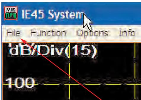
To calibrate your IE-45, tap the "File" menu and select "Input Select." The calibration and input selection window will appear. It contains instructions for calibrating with a calibrator.
