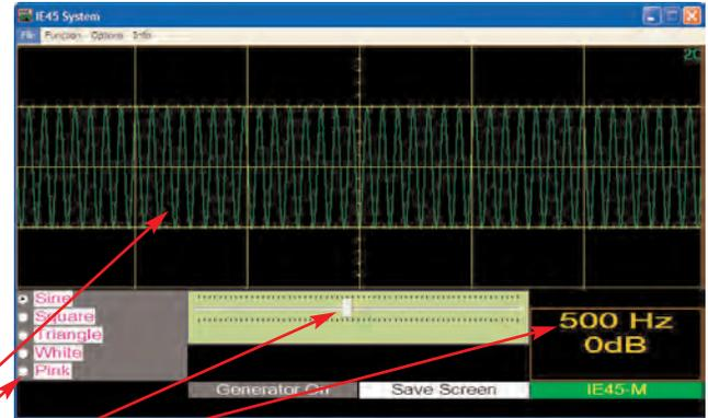
Display of frequency selected by the slider control. The slider controls the output frequency of the Generator.
