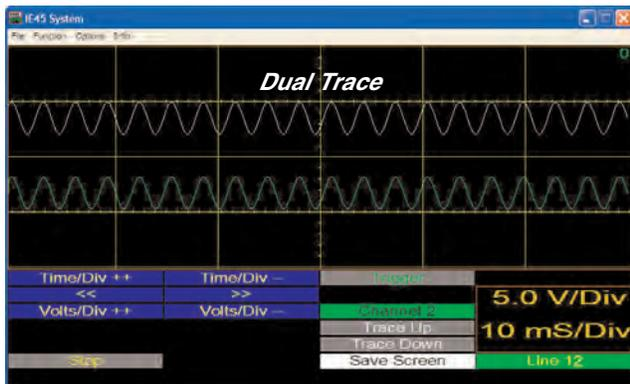
With Channels 1 & 2 Input selected, the "Options" menu allows selection of Dual Trace or XY.
