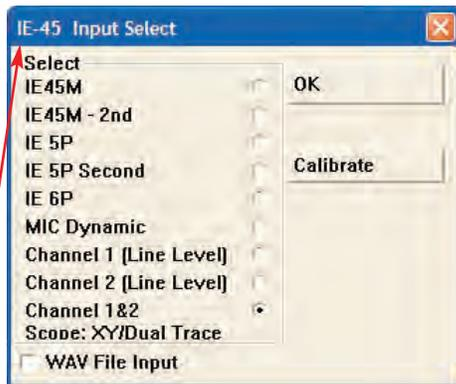
Use "File" > "Input Select" to select line level input(s). For Single Trace Scope, use either Channel 1, or 2 input. For XY/Dual Trace Scope, use "Channels 1 & 2" input.
