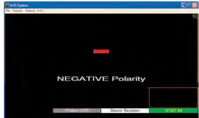
In the example screen above, the IE-45 has “locked” on the signal and identified the polarity of the signal as “Negative.”
