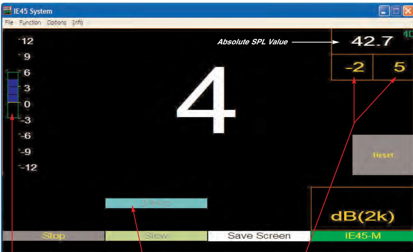
Seat-to-Seat variation is graphically shown by this display. The "spread" is easily viewed and simple to understand.
