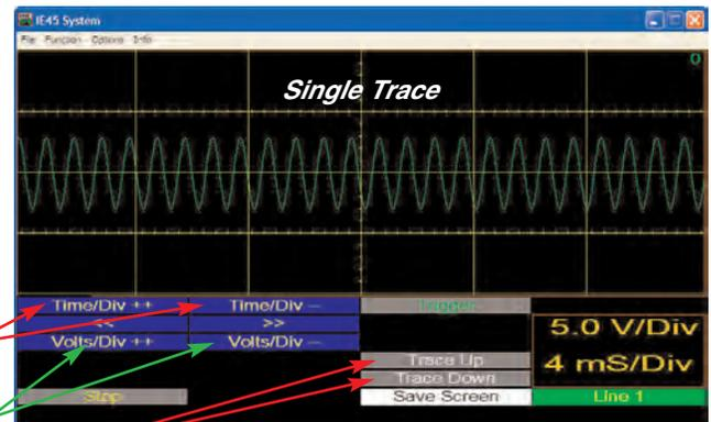
Use these buttons to vertically position the trace on screen. Use these buttons to expand/contract waveform vertically. These buttons expand/contract waveform horizontally.
