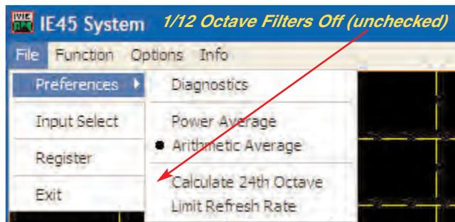
You can activate (check), or disable (uncheck) the 1/12 octave filter set using the “File” > “Preferences” Menu. From this menu, you can also limit (check) the display screen refresh rate. This alone, without disabling the 1/12 octave filters, may be sufficient to improve the performance of some computer systems. As shown below, the 1/12 octaves filters are active, but the screen refresh rate has been limited.
