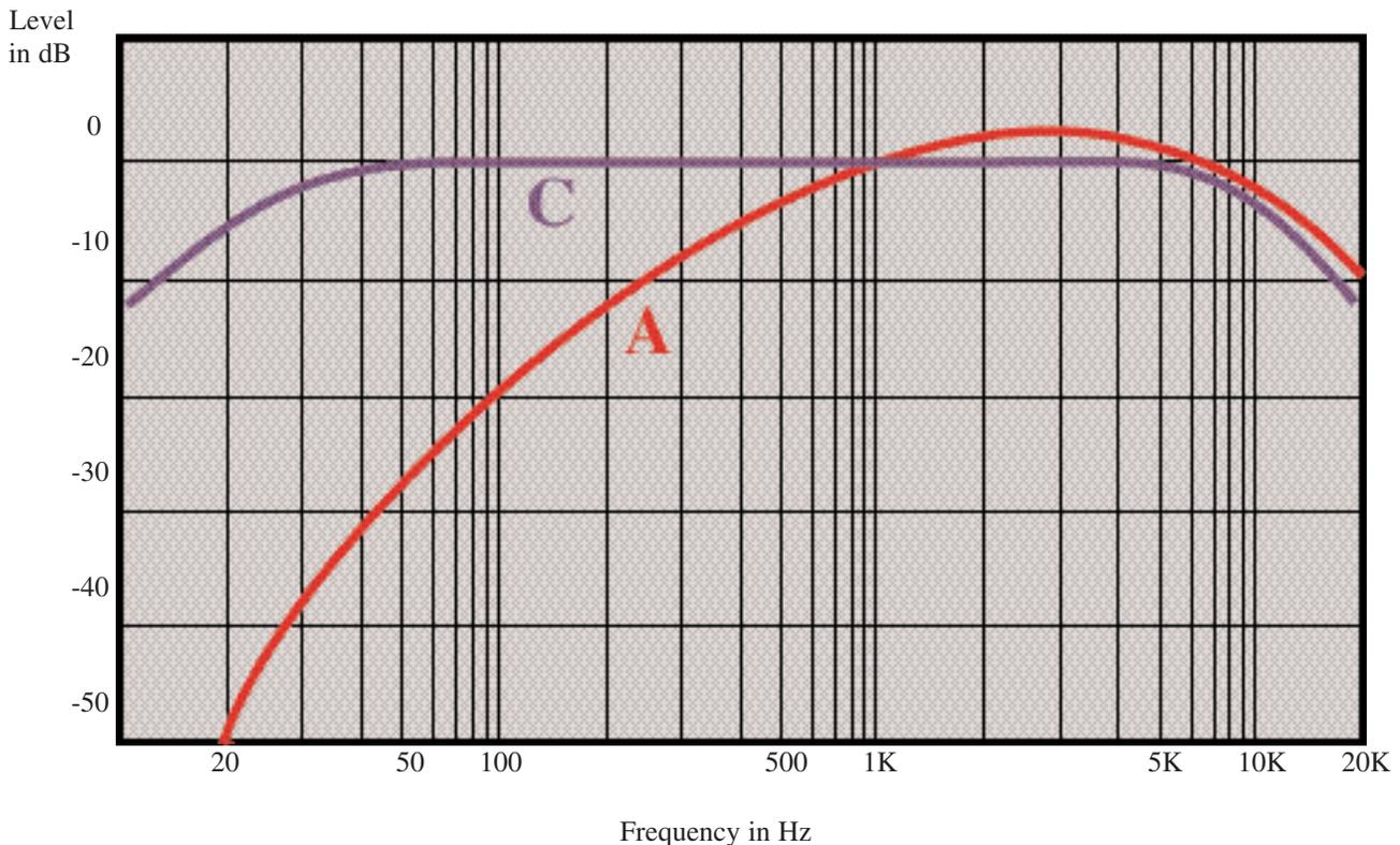
These curves have been integrated into sound level meters for testing sound levels. "A" weighted (dBA) measurements use the "A" curve above, "C" weighted (dBC) use the "C" curve above, and "Flat", or "Z" weighted (dB SPL) measurements use no weighting at all.
