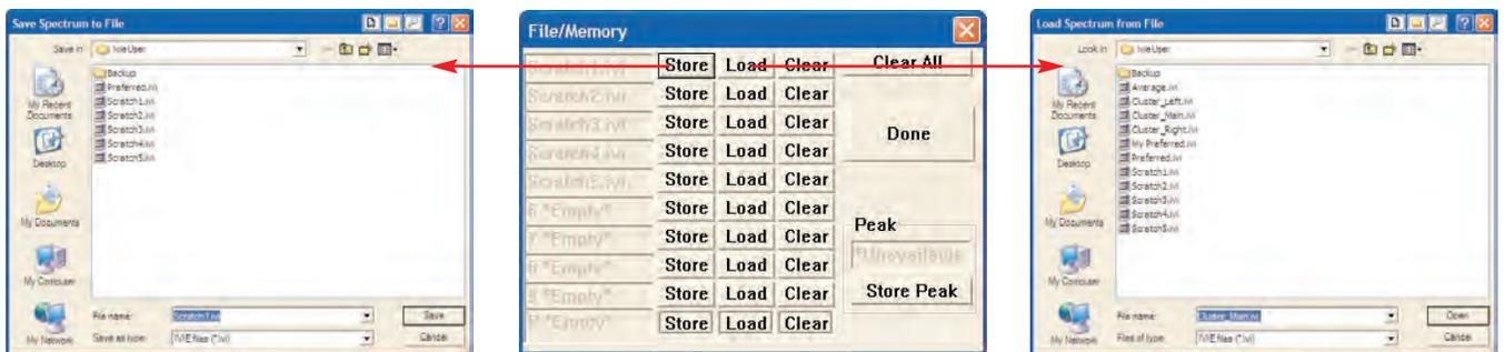
Tapping the red colored "Memory" stylus button brings up the main "Memory Management" window in the center above. From this window, memories can be cleared, stored or loaded. Tapping "Store" brings up the window on the left that allows the storing and naming of memories. Tapping "Load" brings up the window on the right that allows loading memory files from the main memory into the various memory locations such as Scratch memory, Preferred Curve memory or Average memory.
