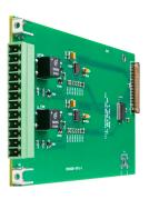
The QUAD-AES IN is a modular digital input card for use with Ivie MAP series devices. Each QUAD-AES IN provides 2 stereo paired channels of either AES3 or SPDIF input on euro-block connectors. Each stereo pair can be individually software configured to be AES3 (balanced or unbalanced) or SPDIF.
