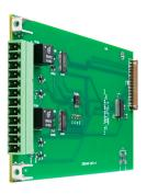
The QUAD-AES OUT is a modular digital output card for use with Ivie MAP series devices. Each QUAD-AES OUT provides 2 stereo paired channels of either AES3 or SPDIF output on euro-block connectors. AES3 (balanced and unbalanced) and SPDIF formats are continuously output on both stereo pairs. Selection of format is made by connection, and No programming is necessary.
