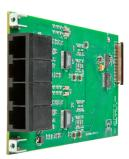
QUAD-TEL is a 4 channel (2 inputs, 2 outputs) modular telephone interface card for use with Ivie MAP series devices. The QUAD-TEL allows a MAP system device to connect directly to standard analog telephone lines. Each channel includes caller-ID decoding, ring detection/validation, DTMF decoding, and call progress tone decoding. Each channel includes a second connector in parrallel for pass through to a telephone.
